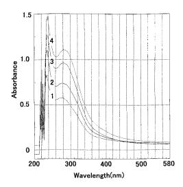
**Figure 1** UV difference spectra of photoirradiated and unirradiated collagen film at different irradiation times: 1, 1 h; 2, 2 h; 3, 3 h; 4, 4 h.
