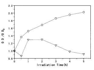
**Figure 7** Changes in optical densities at 280 nm with irradiation time.  $\bigcirc$ , collagen without additive;  $\triangledown$ , collagen containing vitamin E.
