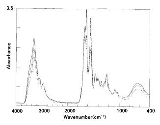
**Figure 3** FTIR spectra of photoirradiated collagen films. Irradiation time, ---, 0 h; ----, 3 h;  $\cdots$ , 6 h.
