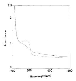
Figure 10 Absorption spectra of collagen containing vitamin  $E \cdots \cdots$ , unirradiated; —, photoirradiated 2 h.
