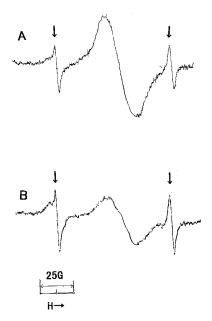
**Figure 5** ESR spectra of photoirradiated (A) collagen, and (B) collagen containing vitamin E. Irradiation time, 4 h. Arrows indicate the signal of  $Mn^{2+}$ .
