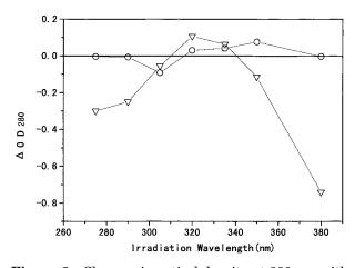
**Figure 8** Changes in optical density at 280 nm with irradiation wavelength.  $\bigcirc$ , collagen without additive;  $\bigtriangledown$ , collagen containing vitamin E.
