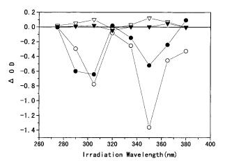
**Figure 9** Changes in optical densities at 1650 cm<sup>-1</sup>  $(\bigcirc, \bigtriangledown)$  and 1550 cm<sup>-1</sup>  $(\bigcirc, \blacktriangledown)$  with irradiation wavelength.  $\bigcirc, \blacklozenge$ , collagen without additive;  $\bigtriangledown, \blacktriangledown$ , collagen containing vitamin E.
