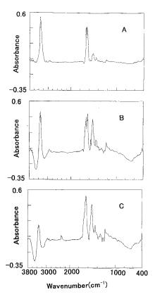
**Figure 11** FTIR difference spectra of thermal-treated collagen (A) at 47°C, (B) at 87°C, and (C) at 117°C.
